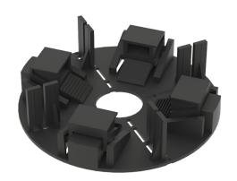
VP-GP has a height range of 24 mm to 35 mm with four independent chocks that may be adjusted in 1 mm increments. Higher heights may be achieved through fixed Extenders of 10 mm, 20 mm, 30 mm and 40 mm in height.
