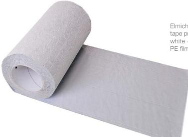
Elmich P50 Sealing Tape is a self-adhesive sealing butyl tape protected by a strong, high density, cross laminated, white crepped polyethylene film. The special crepped PE film allows a 60% elongation/deformability.
